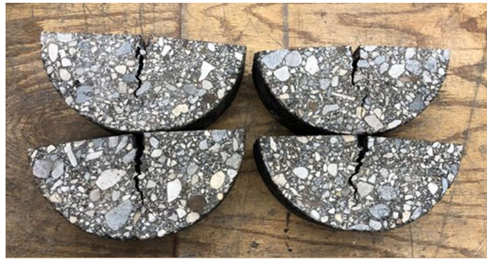
Figure 42. Typical sample after SCB test
