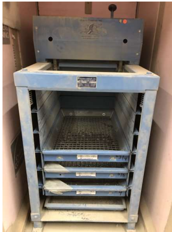
Figure 14. Common set-up of Mechanical Shaker
