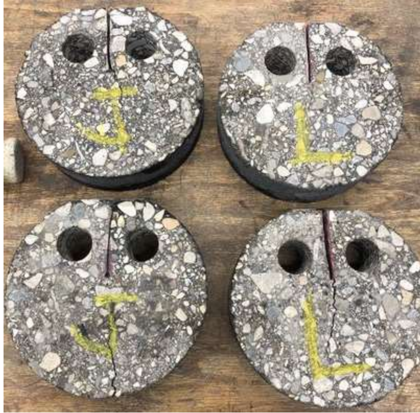
Figure 37. Typical sample after DCT test
