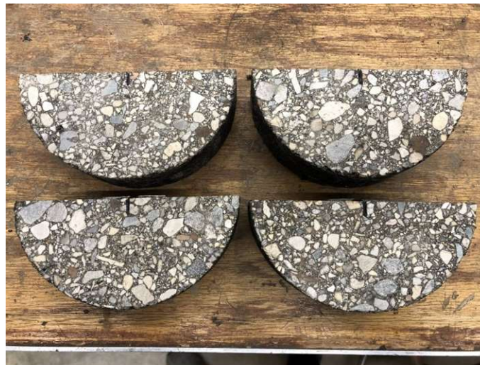
Figure 26. SCB Samples ready for Testing
