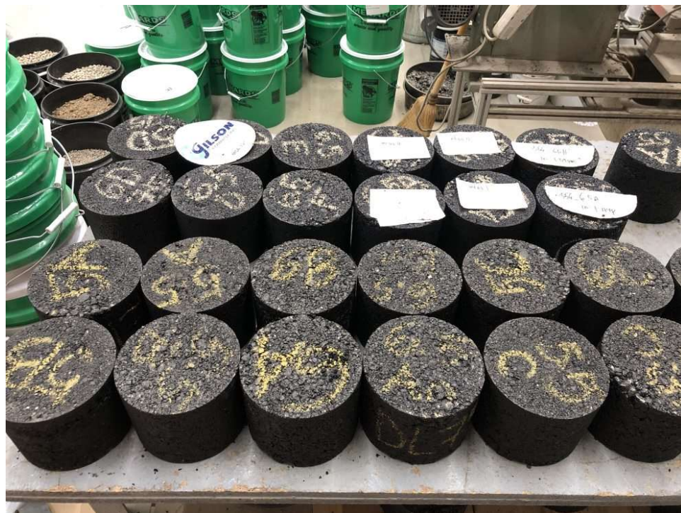
Figure 21. Asphalt Samples ready for G_{sb} Experiment
