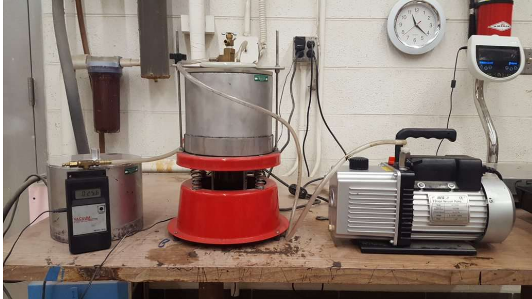
Figure 17. Theoretical Maximum Specific Gravity ( G_{mm} ) Experiment Set-up
