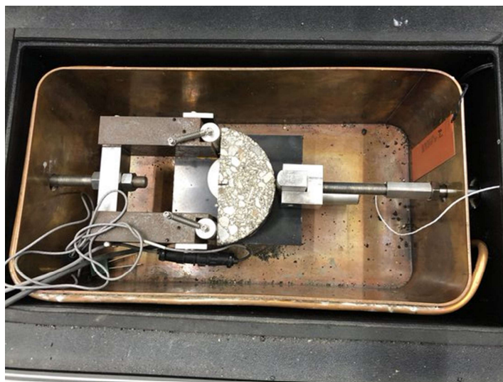
Figure 27. SCB Sample Set-Up
