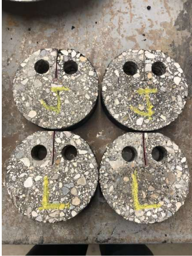
Figure 23. DCT Samples ready for Testing
